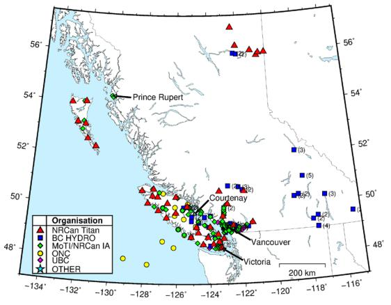
Figure 1. Strong motion seismographs in British Columbia. Numbers in parenthesis indicate the total number of instruments at that site.
