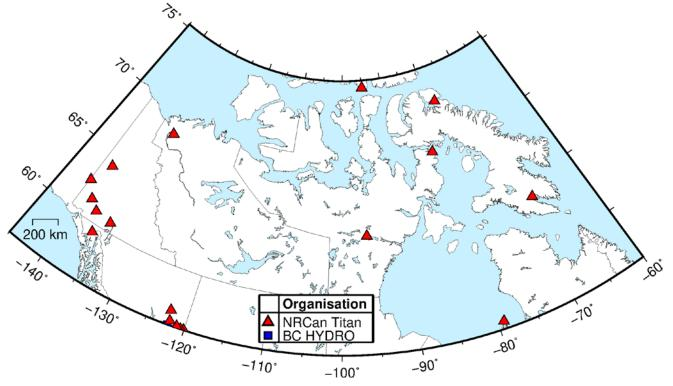
Figure 5. Strong motion seismographs in northern Canada (north of 55°). All NRCan instruments are Titans.
