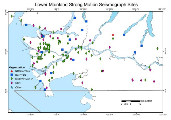
Figure 3. Strong motion seismographs in Greater Vancouver and the lower mainland
